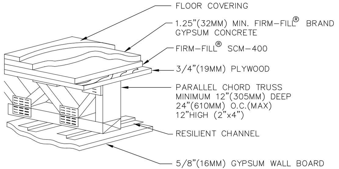
**When installed over open web, 1.25" (32mm) FIRM-FILL® Brand Gypsum Concrete and 3/8" (10mm) FIRM-FILL® SCM-400 achieve excellent fire and sound ratings while providing a superior crack-resistant surface for the installation of finished floor coverings.**
